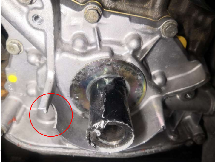
Figure 2 - Grind Slot on Oil Pump Housing
