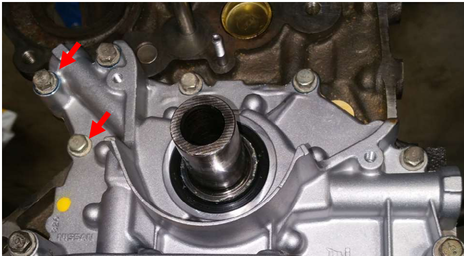
Figure 1 - Remove Bolts on Oil Pump
