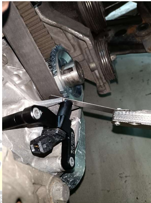
Figure 4 - Setting sensor gap.
