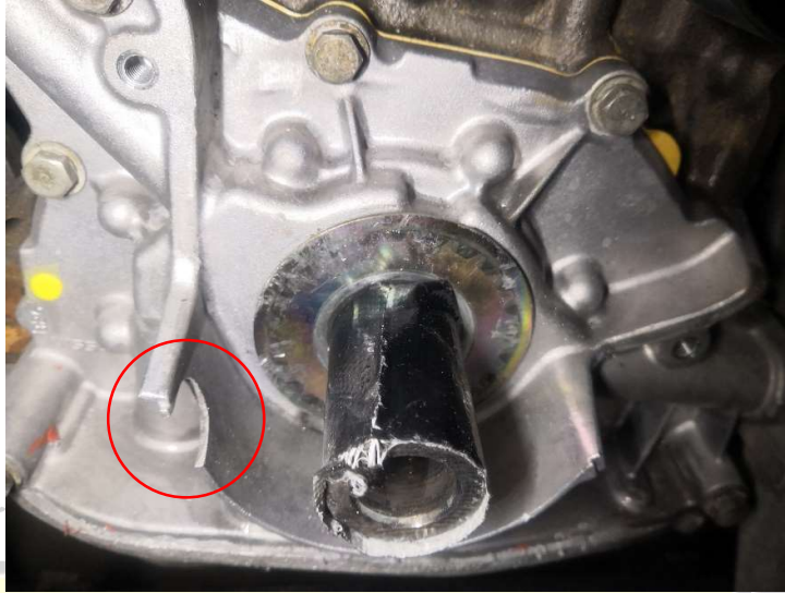
Figure 2 - Grind slot on oil pump housing
