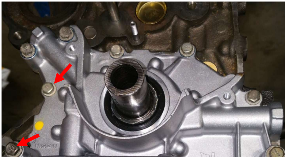
Figure 1 - Remove indicated bolts on the oil pump
