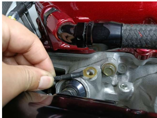
Figure 5 - Connect the ignition sub-harness
