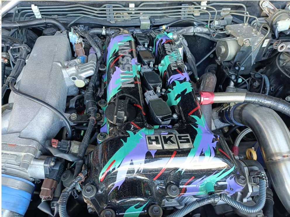
Figure 7 - S15 SR20DET Installation
