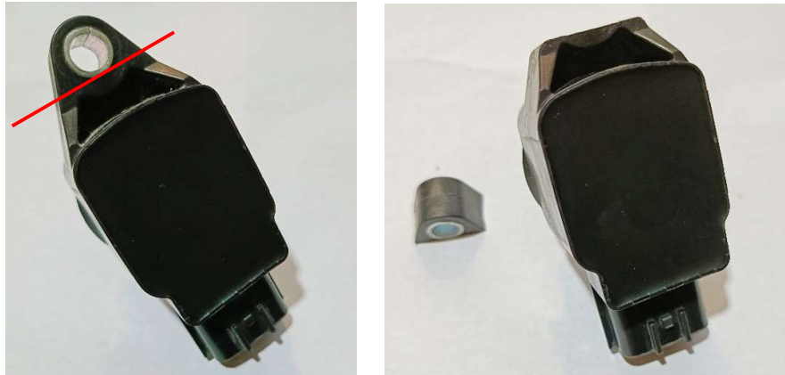
Figure 3 - Cut mounting tab off on one coil for cylinder 1
