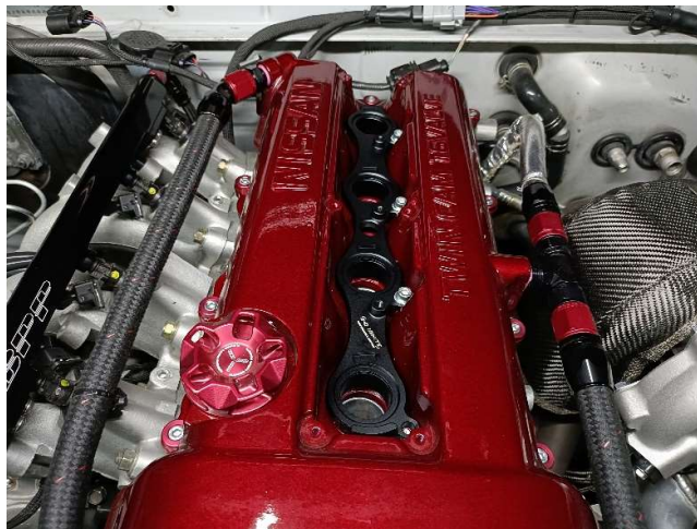
Figure 2 - Install the bracket onto the valve cover
