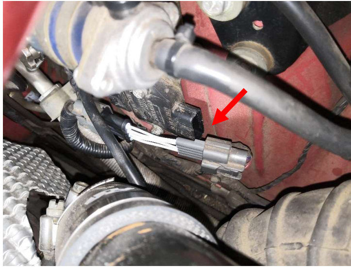
Figure 8 - Connect igniter patch harness
