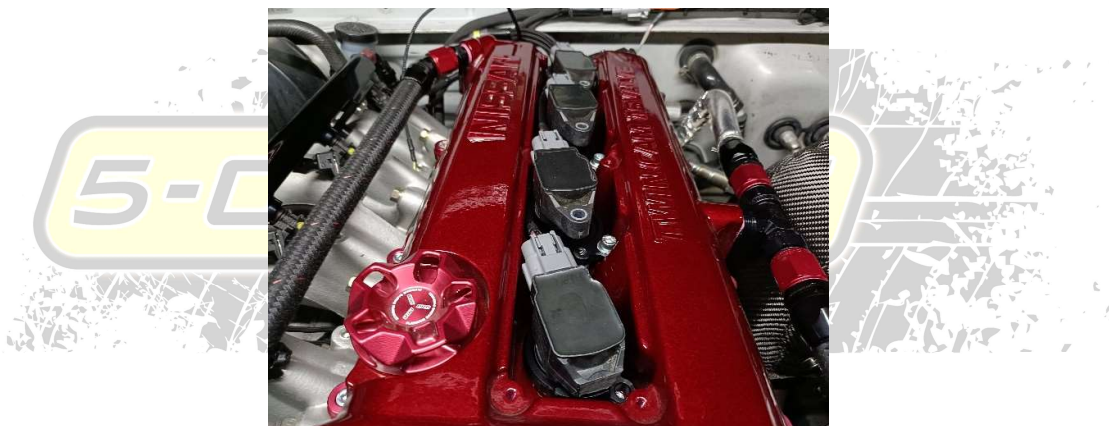
Figure 4 - Fit the coils onto the engine
