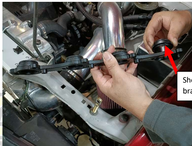
Figure 1 – Install the sealing boss onto the mounting bracket
