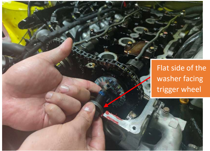
Figure 7 – Apply Medium Loctite On The Thread
