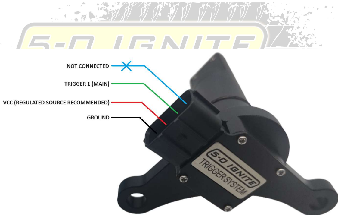
Figure 14 – 5-0 Ignite SR Cam Trigger V3 Sensor Pinout
