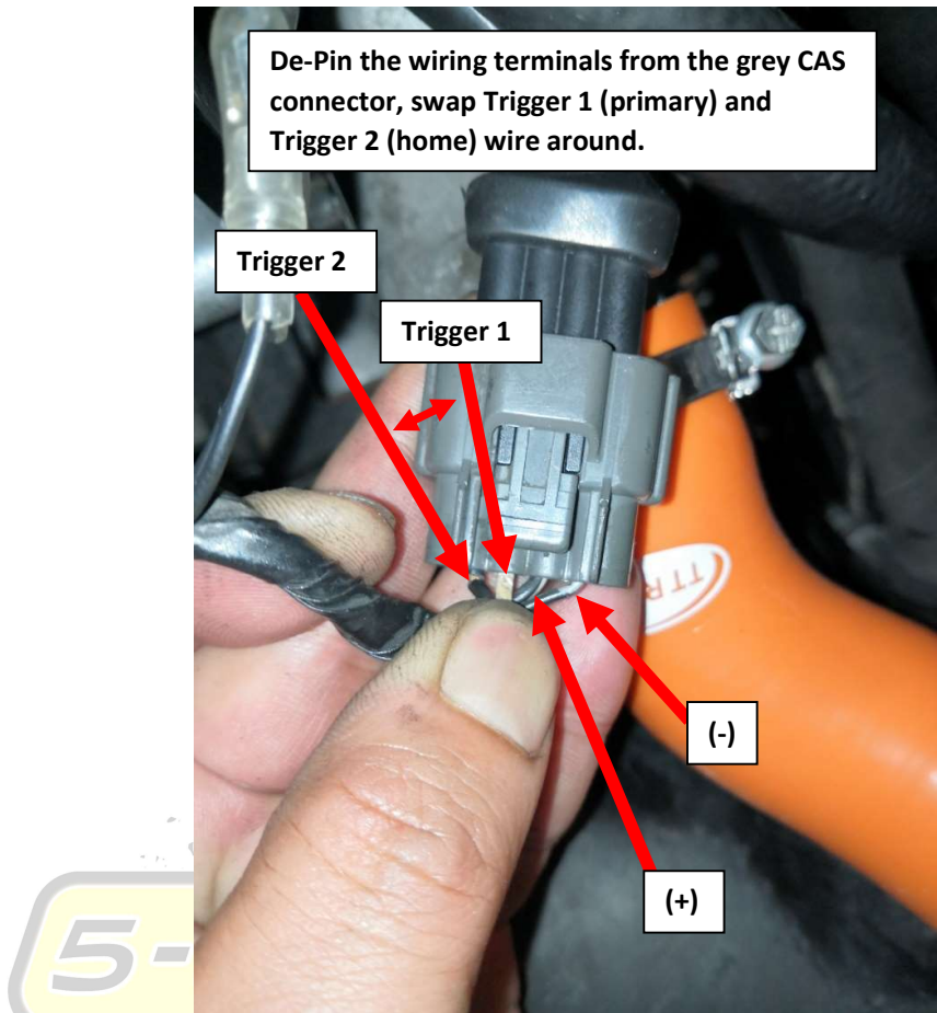
Figure 15 - Swapping Trigger Wires Around (Required on Some ECUs)
